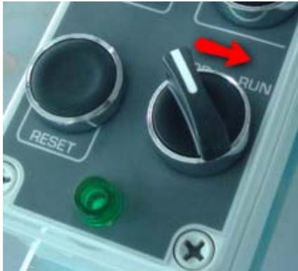
A low pitched squeak can be heard as the frequency inverters synchronise with the motors (this is normal). The Grinder should not start operating. If this happens switch back to **STOP** and check the process again.
