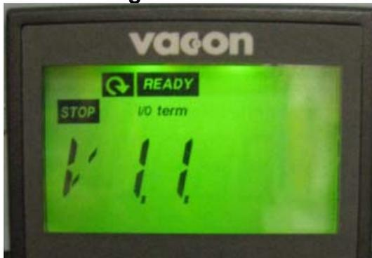
Press **Right** once more to display the "Output Frequency" as displayed by "**Hz**"
